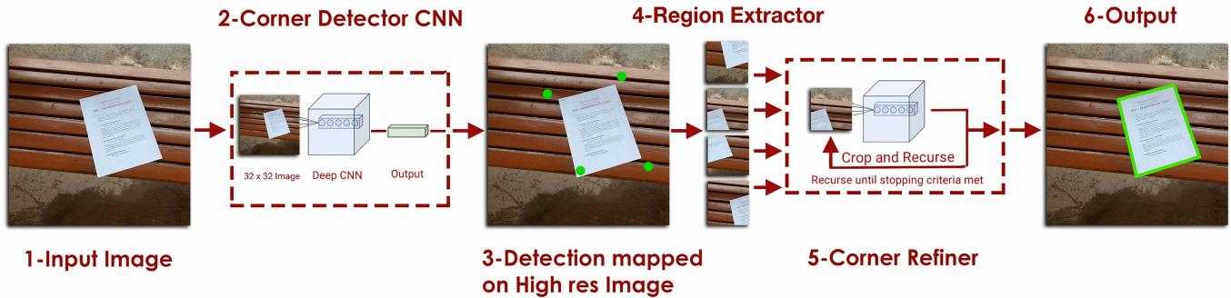
Fig. 1: Overall architecture of the system. 32 x 32 Image is used by Corners Detector to predict four corners. This prediction is used by region extractor algorithm to extract corner images. Each of the four corner images are then recursively refined by Corner Refiner to get the final output.
